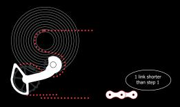
STEP 2: When tension is applied on the chain and the OSPW X System appears to be aligned as the diagram above, the chain needs to be cut (1 link shorter than step 1) and connected by the required amount of links in order to achieve sufficient tension in this gear combination (always the small cog on the cassette).
