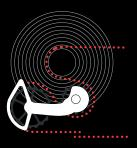
STEP 1: Place the chain on the smallest cog on the cassette. To find the correct chain length, pull the two chain ends together, just as you would when needing to cut a chain to length. The lower part of the cage should start to move downwards, away from the cassette, as referenced in the second image.
